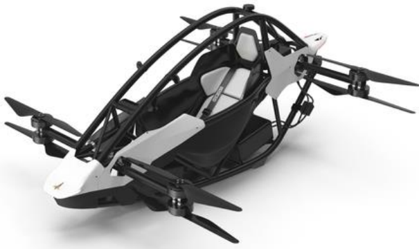
Fig. 2. Empty model of Jetson One [5]
