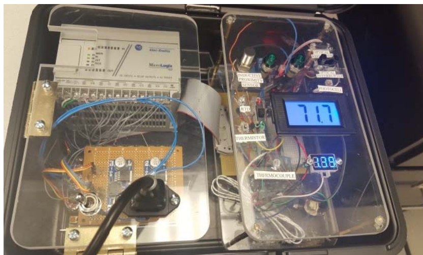
Figure 2. Diagram and Photo of Portable PLC Kit Layout (with Sensor Module).
