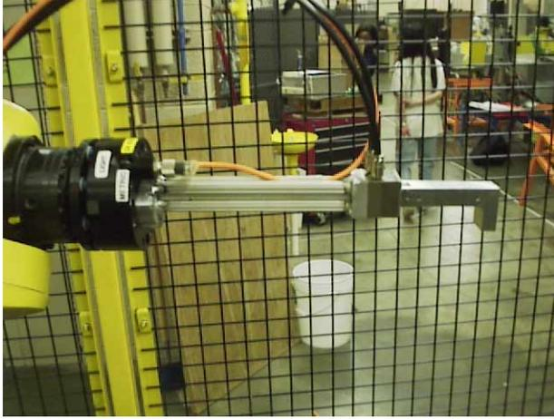
**Figure 4. Robot EOAT**
