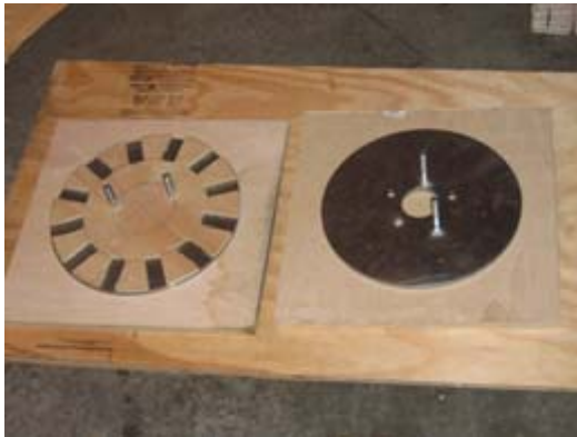
Figure 3. Rotor plates with magnet guide
