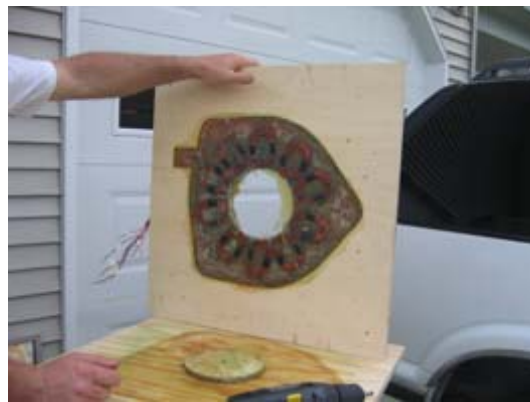
Figure 2. Stator after resin poured and dry
