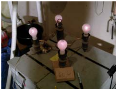
Figure 9. Testing the output through four light bulbs.
