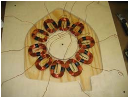
Figure 1. Wound coils in stator mold
