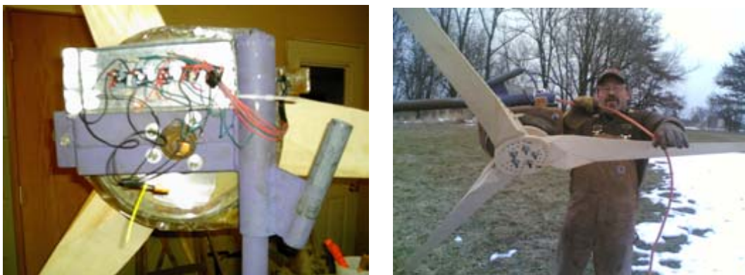
Figure 8. Blade assembly for the Axial Flux Wind Turbine
