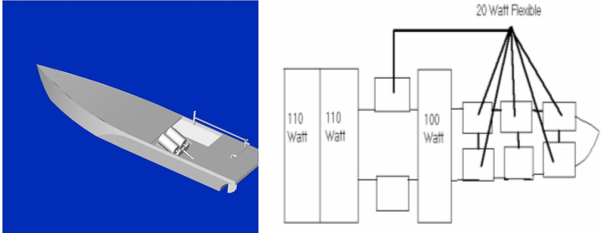
Figure 1. Initial ProE Design of solar-electric boat hull and placement of PV modules.
