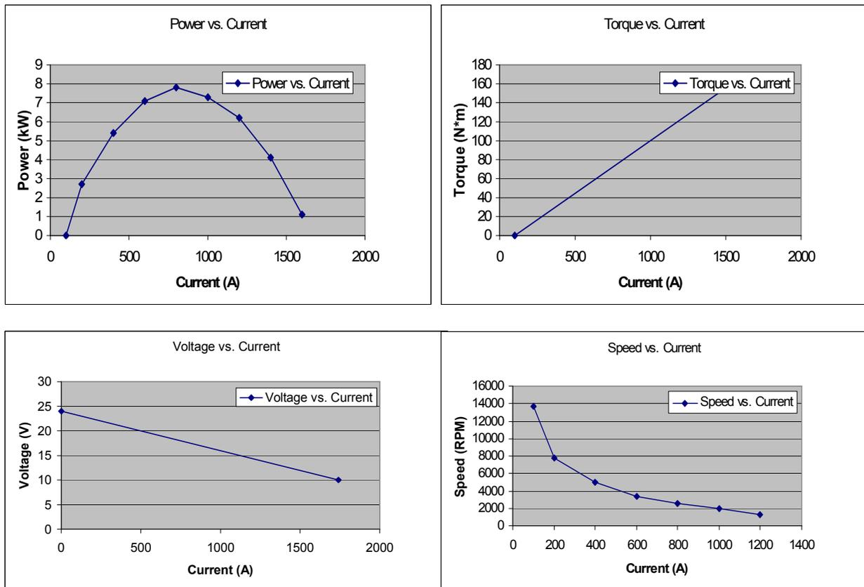
Figure 3. Electric Power, Torque, Voltage, Current, and Speed Characteristics for the motor
