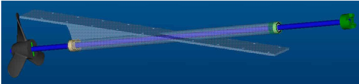
Figure 6. Three -dimensional model of new output shaft
