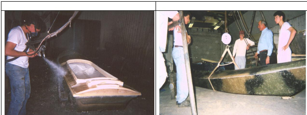
Figure 2. Fiber-glass Hull Manufacturing
