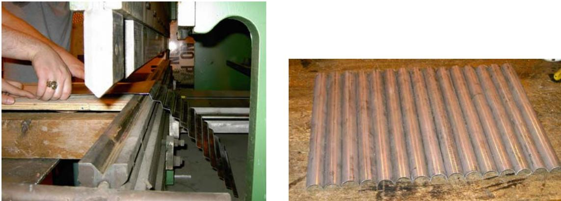
Figure 5. Fabrication of corrugated surface<sup>19</sup>
