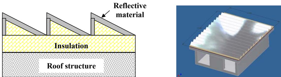
Figure 1. Basic passive cooling system design<sup>19</sup>
