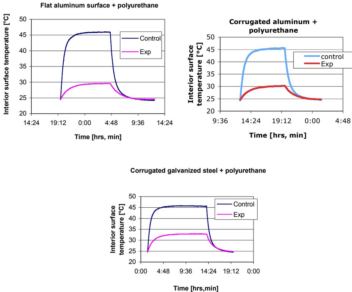
Figure 8. Interior surface temperatures of houses for three passive cooling system prototypes<sup>19</sup>
