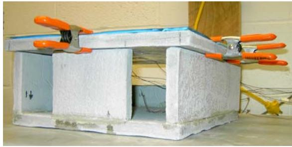
Figure 6. Assembled passive cooling system<sup>19</sup>
