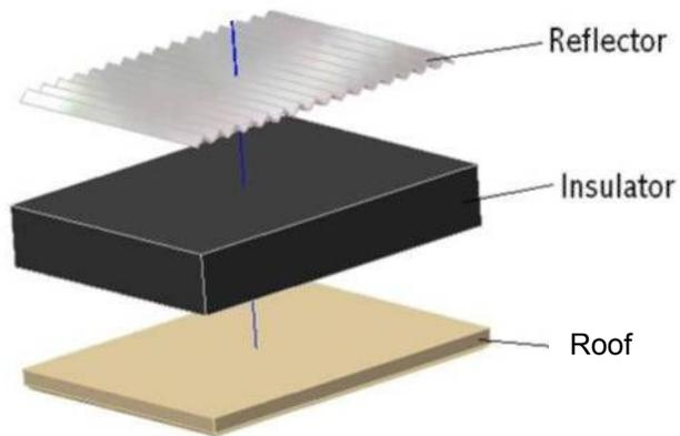
Figure 4. Passive cooling system prototype<sup>19</sup>
