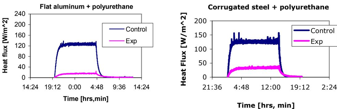
Figure 9. Heat flux measurements of optimal passive cooling systems<sup>19</sup>
