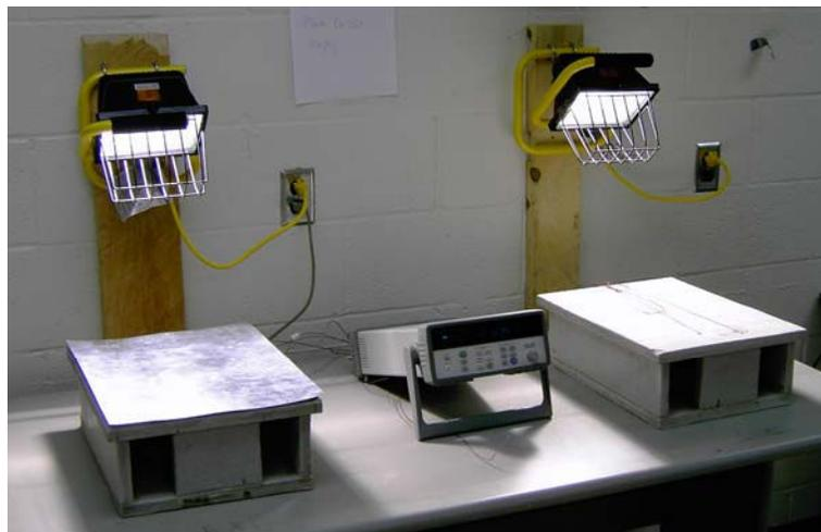
Figure 7. Control and experimental houses under 600-W lamps<sup>19</sup>
