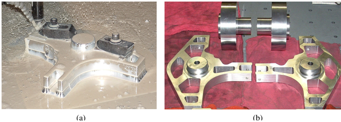
Figure 4. Lower A-arm Machining and Assembling into Chassis, (a) Part stock (b) machined arm cap (c) assembly fixture (d) A-arm in the chassis
