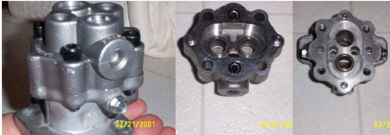
Figure 1. A Danfoss hydraulic gear pump was used for the project
