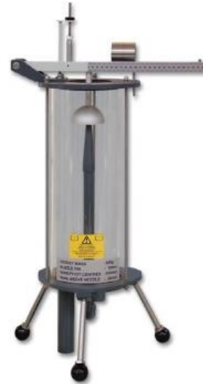
Figure 2. Impact of a jet experiment unit from TQ equipment
