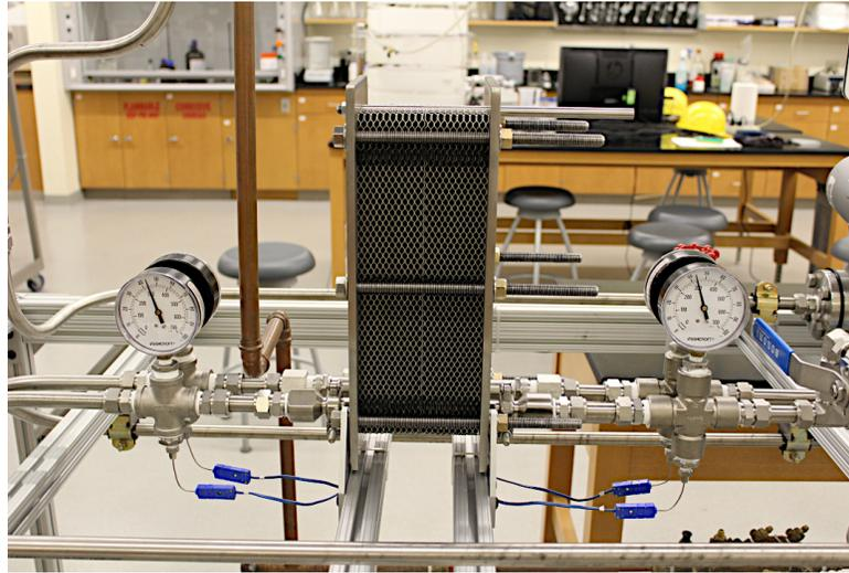
Figure 10: View of plate heat exchanger. PCW thermocouples (near side) and HHW thermocouples (far side) are visible
