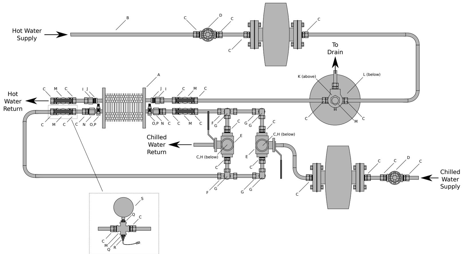
Figure 3: Detail of PHX assembly (top view). Labels reference Table 1.
