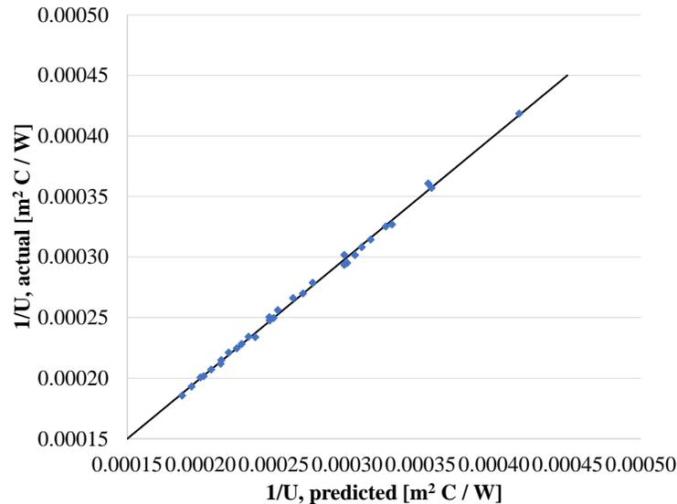
Figure 9: Actual vs predicted values for  $1/U$ , counter-current
