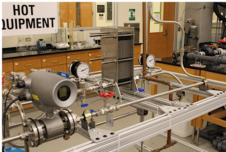
Figure 12: View Showing HHW flow rate adjustment valve and flowmeter.
