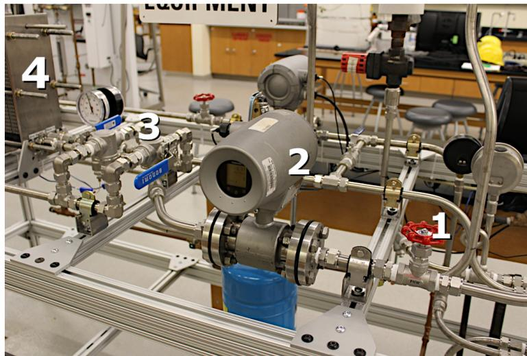
Figure 11: View Showing (1) PCW flow rate adjustment valve, (2) PCW flowmeter, (3) three-way valves for controlling PCW flow direction, and (4) plate heat exchanger
