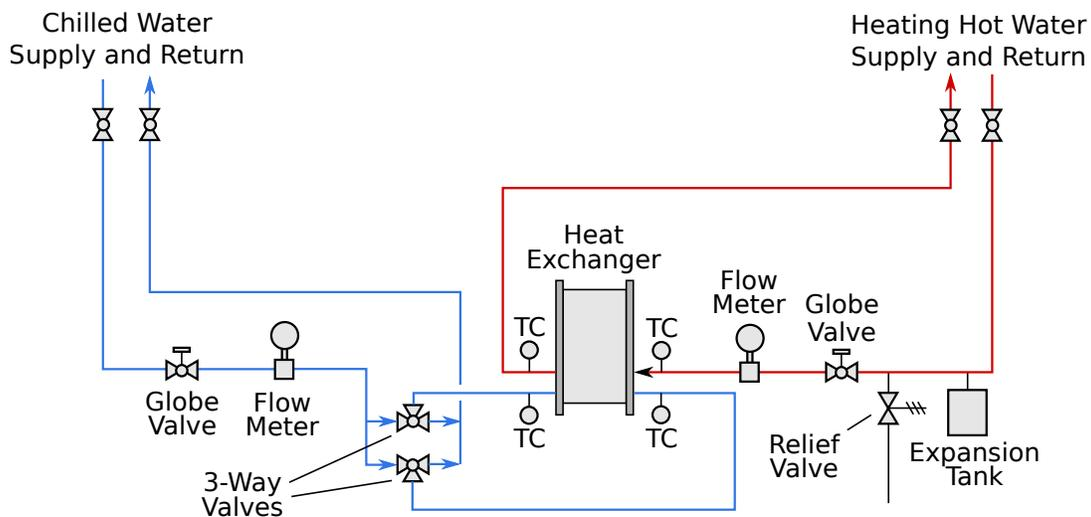
Figure 1: Initial Process Flow Diagram of PHX
