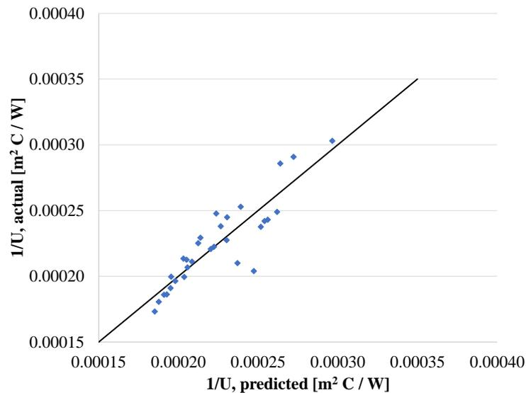
Figure 8: Actual vs predicted values for  $1/U$ , co-current
