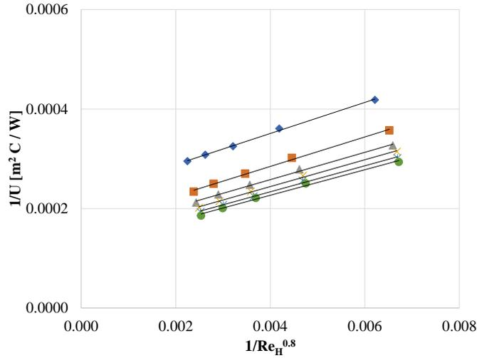
Figure 6: Wilson Plot for counter-current configuration
