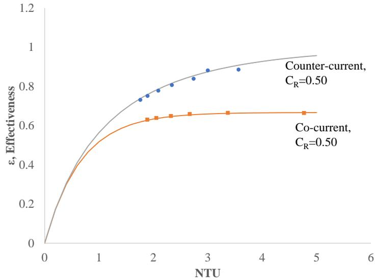
Figure 7: NTU vs Effectiveness for Co-Current and Counter-Current Flow with  $C_R = 0.5$ . Curves show theoretical values, points show experimental values
