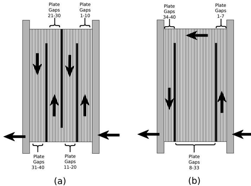
Figure 4: Original four-pass plate arrangement (a) and modified plate arrangement (b)
