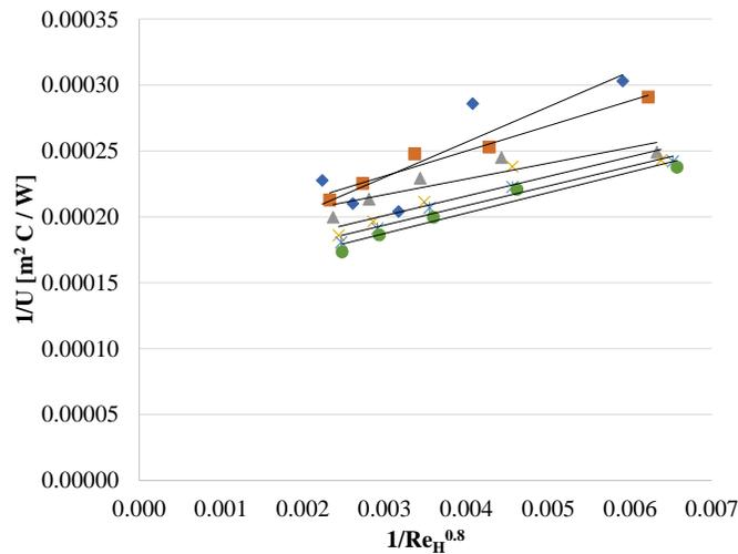
Figure 5: Wilson Plot for co-current configuration
