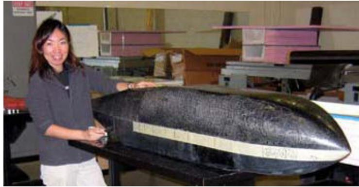
Fig. 7 A CNC-machined foam mold and the thin, light carbon-epoxy fuselage
