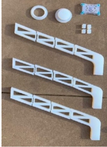
Figure 10. Assembly of the 3-D Printed Drone Legs
