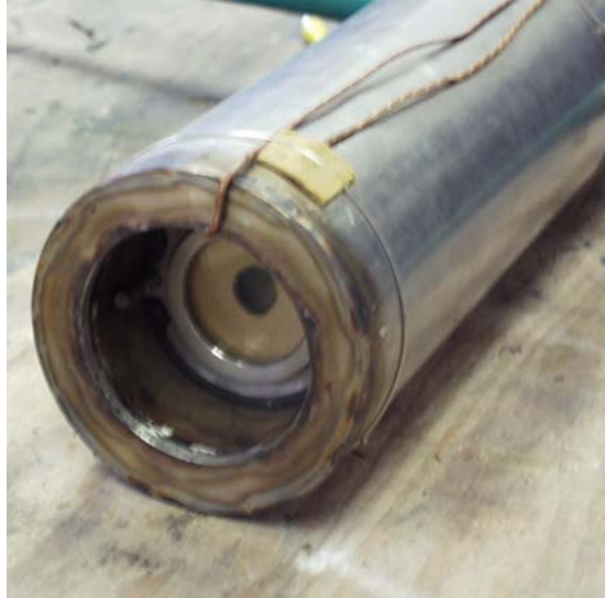
Figure 5. Camera Housing with Thermocouples.
