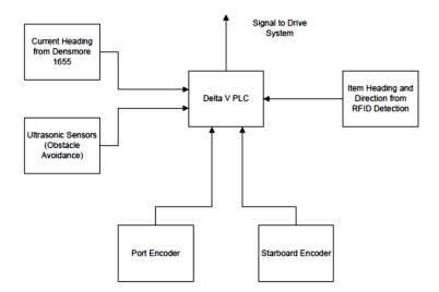
Figure 2 Navigation System Block Diagram
