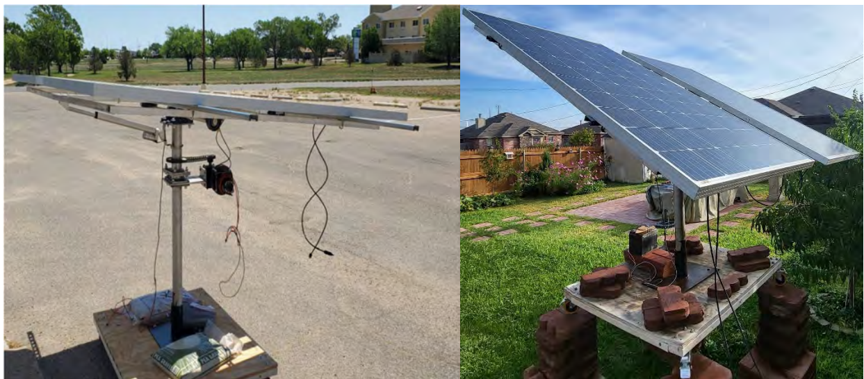
Figure 2. Solar PV prototype with dual axis Sun tracking capability
