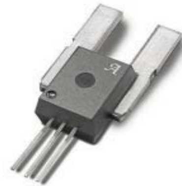
Fig. 12. The Allegro Microsystem ACS758 current sensor [Courtesy of the manufacturer].
