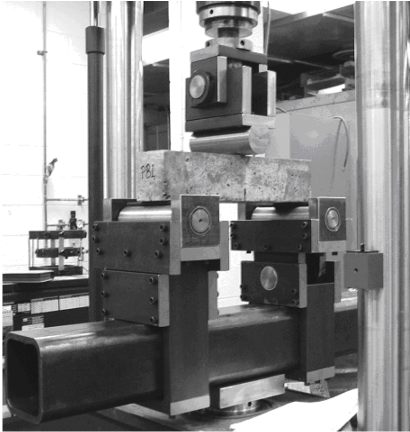
Figure 3: Three-Point-Bend Test Setup
