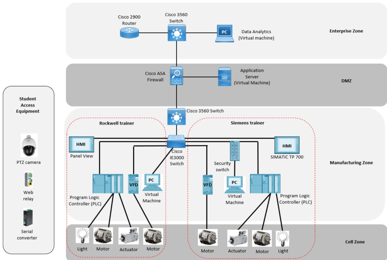
Figure 2. CPwE lab pod design as it aligns with the four CPwE zones.
