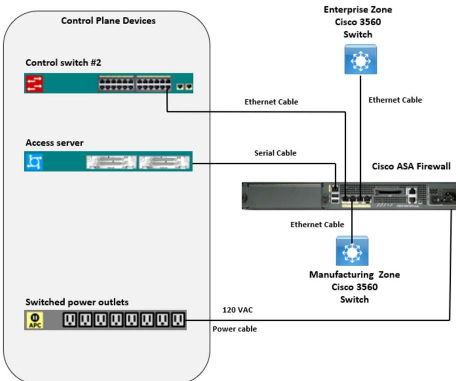
Figure 4. Detailed view of control plane and lab pod connections to the Cisco ASA firewall.
