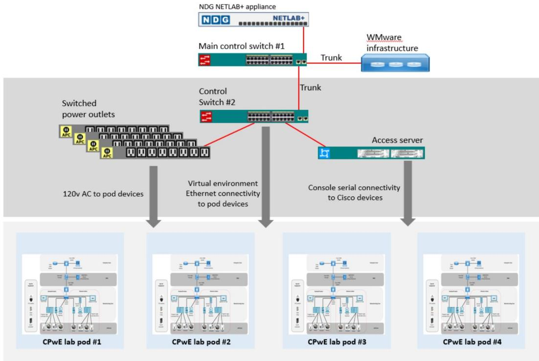
Figure 3. Control plane infrastructure required to support four CPwE lab pods.
