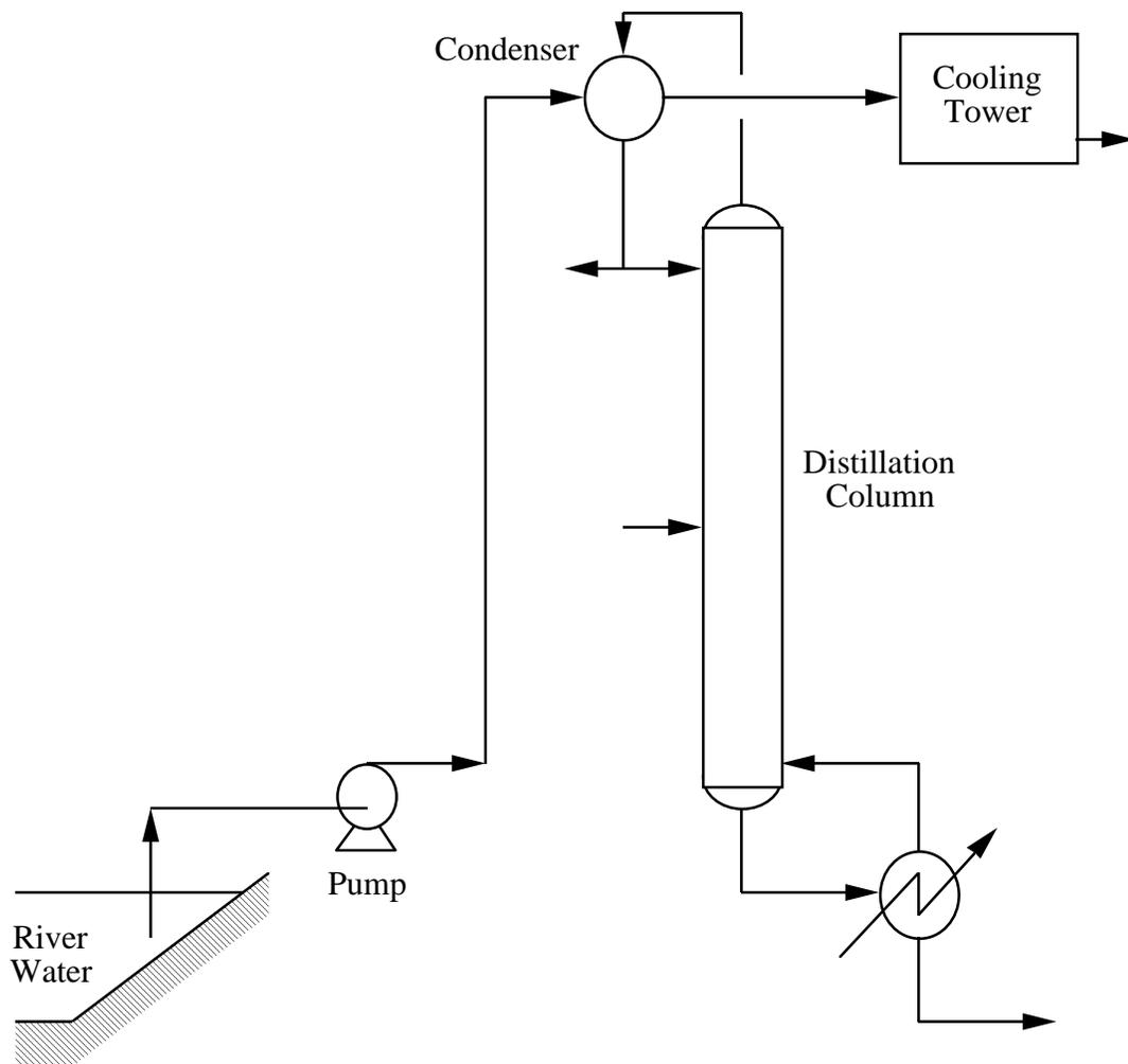
Figure 1. Schematic diagram of one portion of the ethanol case study.
