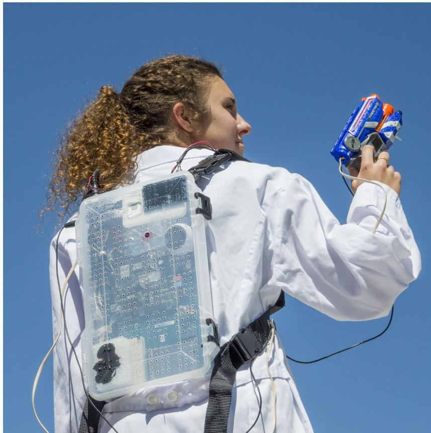
Figure 2: Laser-Tag System Worn By Student
