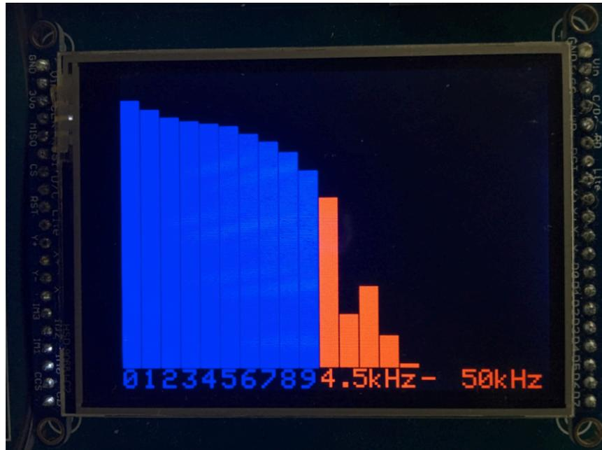
Figure 5: FIR Filter Response Plotted on the TFT Display
