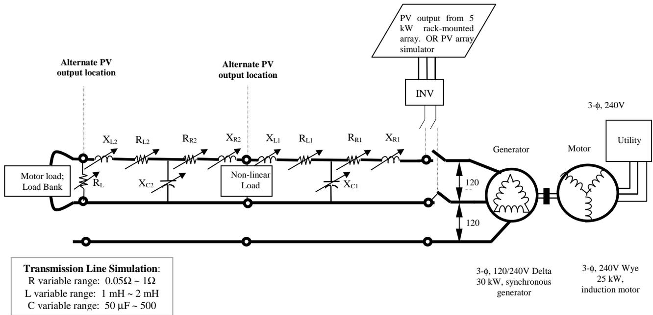
**Fig. 1. A schematic of the lab setup**
