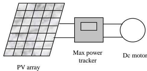
**Fig. 5. Direct dc motor operation with PV**
