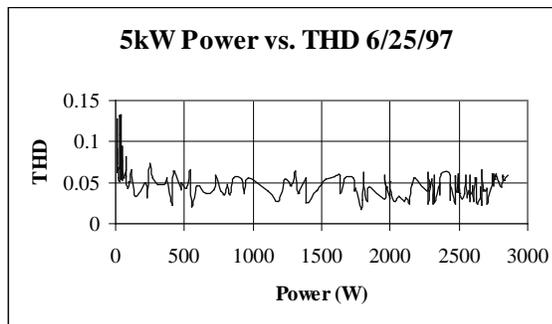
**Fig. 3b. Total harmonic distortion from PV inverter connected to utility.**
