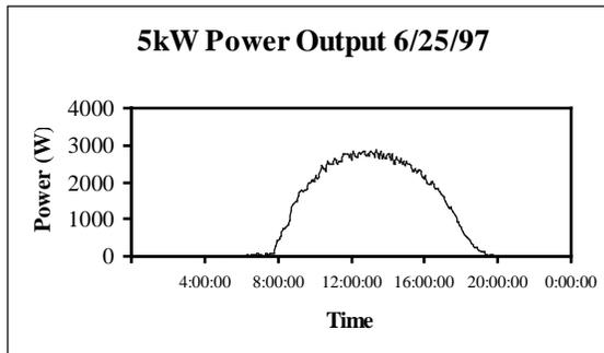
**Fig. 3a. AC power output from a 5 kW PV system.**
