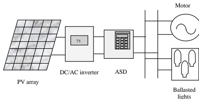
**Fig. 4. PV in the presence of Non-linear loads**
