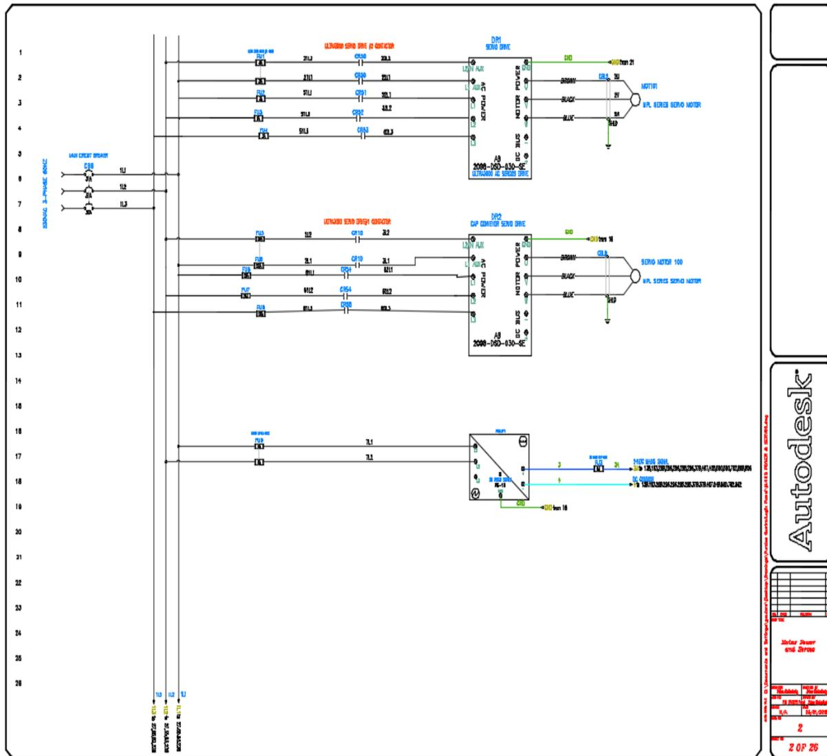
**Fig 4: Main Power Diagram of Ultra 3000 Servo Drive in The Trainer Panel**
