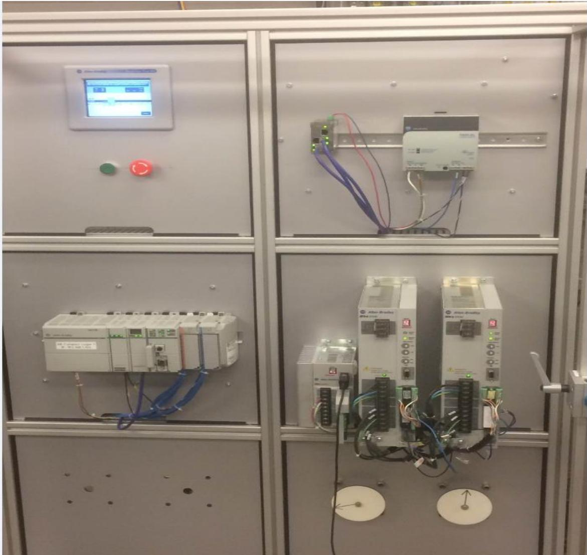
**Figure 3: Real time PLC Laboratory Trainer Panel**
