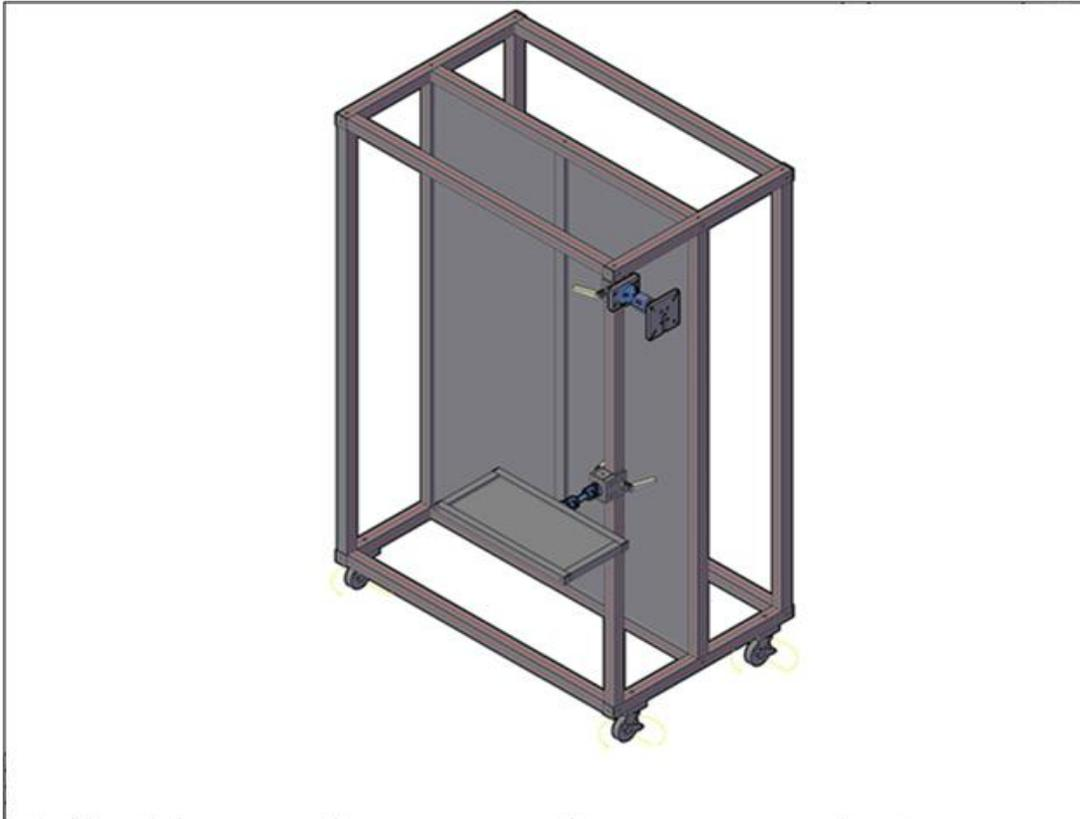
**Figure 2: 3D Design (Preliminary) of the Trainer Panel.**
