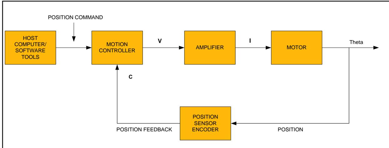
**Figure: 1 Servo Motor Working Principle**
