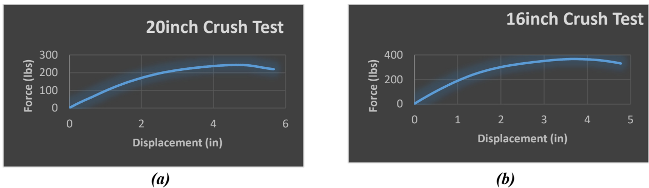
Figure 1: (a) Force vs. Displacement curve for 20-inch alucore; (b) Force vs. Displacement curve for 16-inch alucore
