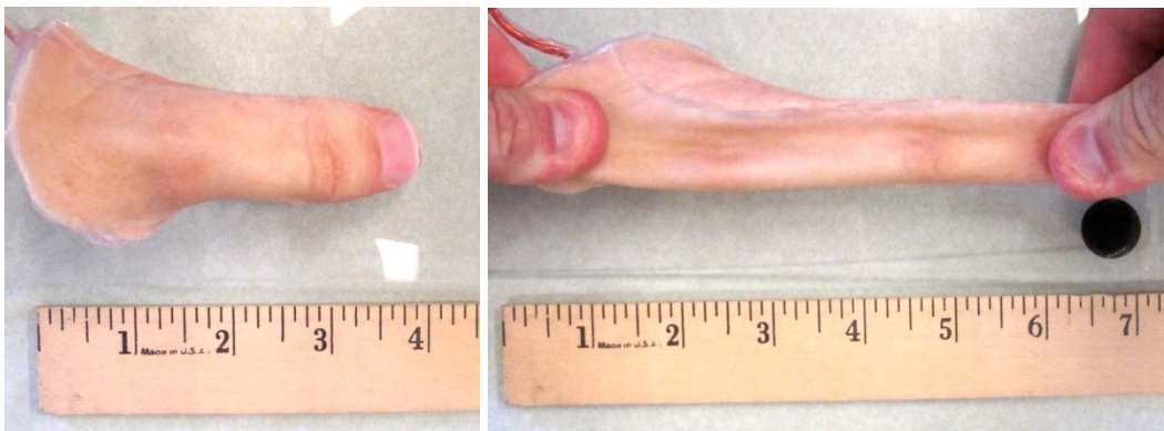
Figure 12: The thumb prototype is stretched 75% without damage.
