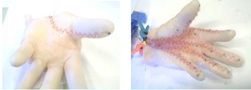
Figure 4: Embedding of sensors onto the prototype skin. Zigzag wire connections were used to allow the stretching and deforming of the skin sensor.
