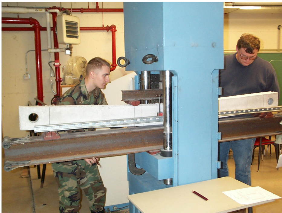
Figure 2: Three-point Load Test on a Simply Supported Reinforced Concrete Beam
