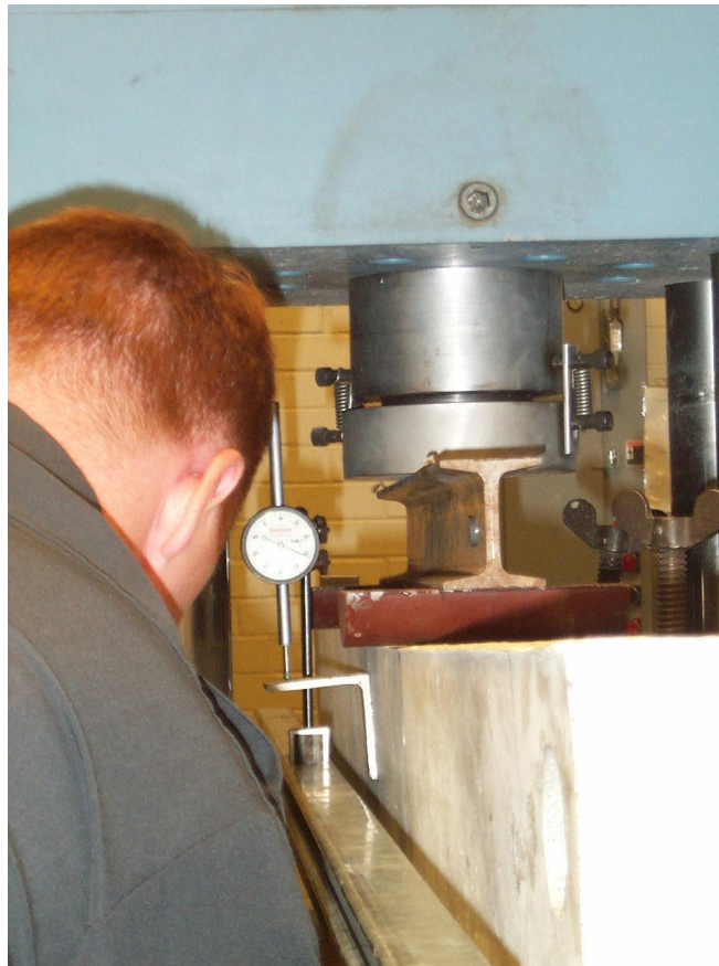
Figure 3: A Dial Gage is Attached to the Center of the Beam to Measure Deflections
