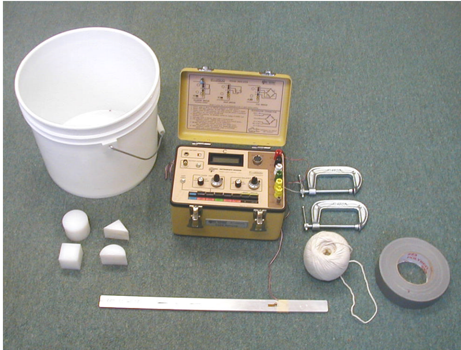
Figure 1: Equipment for Beams in Bending Laboratory
