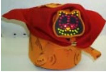
**SuperG.** This Garfield robot can talk and sing. Its special face built using LEDs is mounted on a servo-motor, along with its moving tail. Both are used to express the mood of the robot. Contact switches are used to pet the robot. When happy, SuperG also starts to purr. A keyboard placed under the cape is used to select different behavioral configurations. By clapping, the robot could also be directed to move or to stop.
