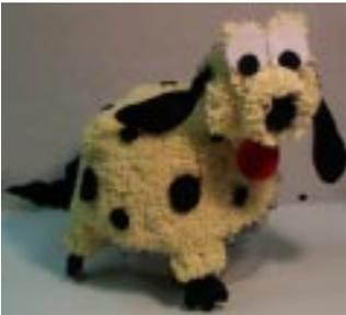
**Robus-T.** This robot-dog has a pyroelectric sensor in its nose to move toward people. Touch buttons are also installed on its back to interact with the child. The head and the tail move using servomotors, and are used to express the mood of the robot.
