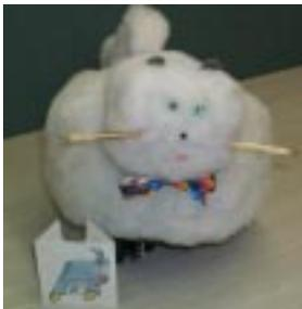
**Diskcat.** This robot has a special fur exterior and looks like a cat. Games like ‘Simon says’, dancing and visual effects using LEDs as eyes and on the back of the robot have been implemented. Resistive bend sensors are used as whiskers.
