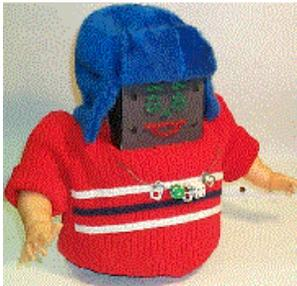
**TOM.** This robot is designed to portray a hockey player robot, build to resist hard usage, because one profile indicated that a child had special interest in hockey. It also has a face made of LEDs and two arms mounted on servo-motors. The robot can play music, dance, move around and say the name of some hockey players when the child pushes some buttons in the proper sequence.
