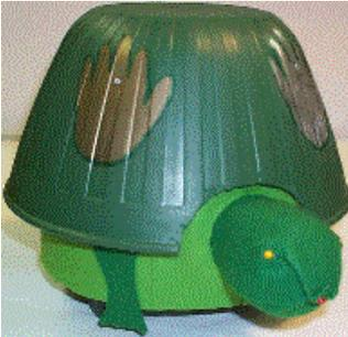
**Paradigmes Proactifs.** This turtle uses LEDs to illuminate its eyes and mouth, and photoresistors to detect that the child is touching its shell at the appropriate places, generating distinct sounds. The robot can dance, play music and race with the child. Special care is made to make the robot robust to hard interplay conditions.
