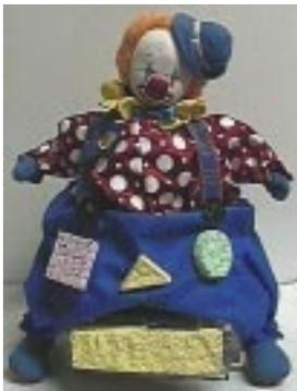
**CARI.** This robot-clown asks the child to play to three different games: to dance, to press on the round, the triangular or the square shape push buttons, or to pursue the robot. The head of the robot is mounted on a servo-motor and eyes are made with green LEDs. The legs of the robot are attached to the wheels to go up and down when the robot moves.
