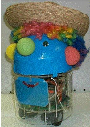
**M<sup>3</sup>.** This clown is programmed to call the name of the child as it moves. It can dance and play with the child using its nose and ears to interact. It smiles or shows signs of sadness depending on the situations. At the end the robot can give some candy to the child by opening its mouth, made using a CD-ROM reader.
