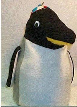
**TOBY.** This penguin can follow a light source and when it detects a loud noise, the propeller on top of its hat starts to turn. Clapping is used to start the robot. The robot also comes equipped with a console used in a game where the robot asks the child to correctly identify an object. Students in this team also found a way to improve the sound generation device.
