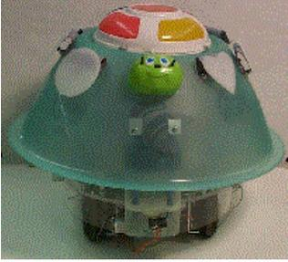
**Kiss.** This robot-turtle offers different games based on shape recognition and dances when the child succeed. It also uses small motors and a mechanism<sup>ii</sup> to make the shell move.
