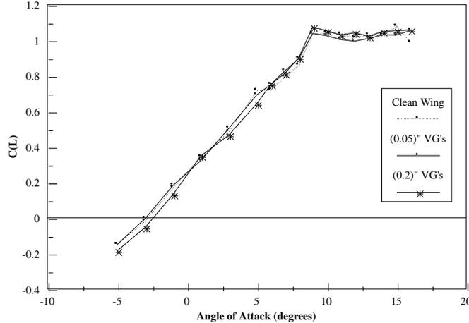
Figure 4: Comparison of Lift Enhancement Using VG's of Different Heights<sup>2</sup>
