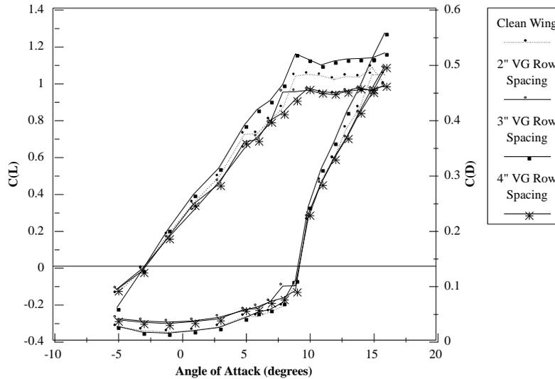
Figure 5: Influence of Spacing Between Adjacent Vortex Generators<sup>2</sup>
