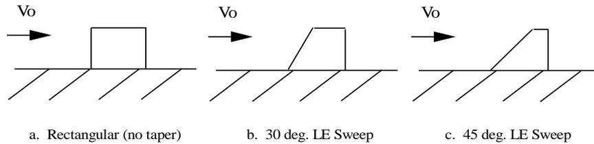
Figure 2: The 3 VG planforms tested.
