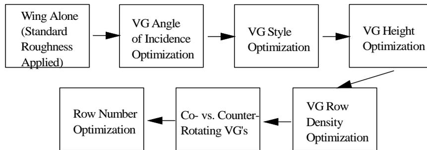
Figure 3: Basic VG optimization test procedure<sup>2</sup>.
