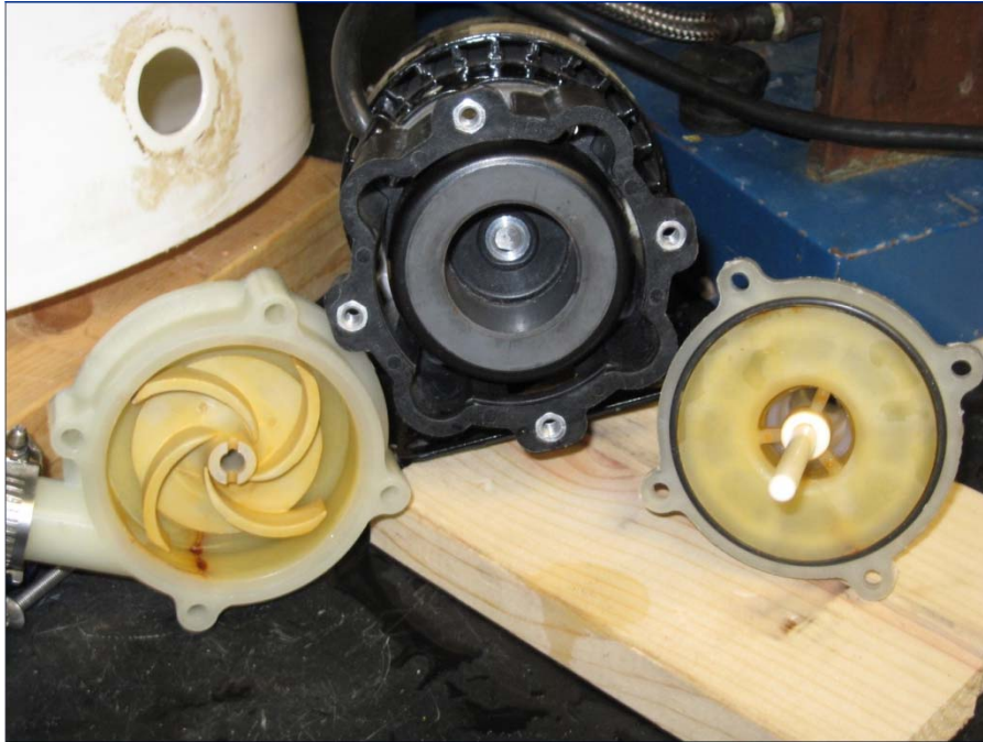
Figure 3. Photograph of the Disassembled Pump
