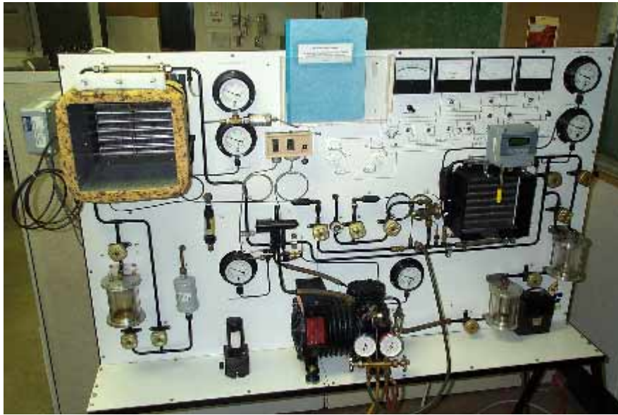
Renovated Refrigeration Trainer
