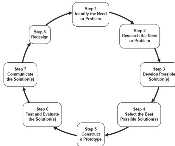
Figure 1: The engineering design process.<sup>[10]</sup>
