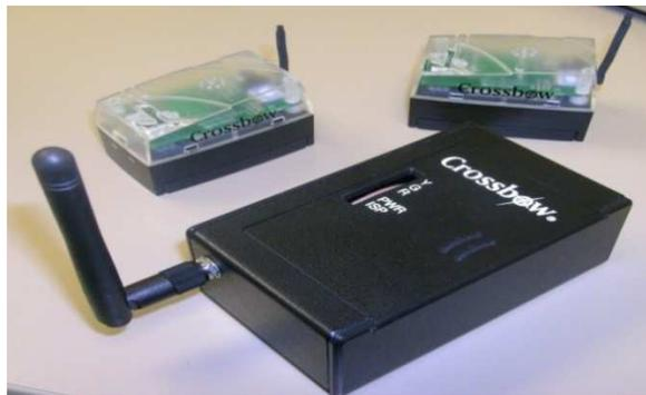
Figure 1. Starter Kit (two wireless nodes and one base station)
