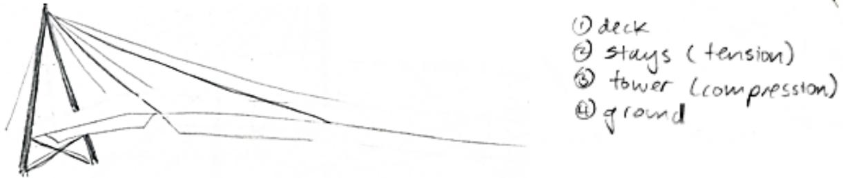
**Figure 4.** Drawing of the Sabrina Footbridge limited to approximately fifteen lines. Drawing courtesy of Demi L. Fang.
