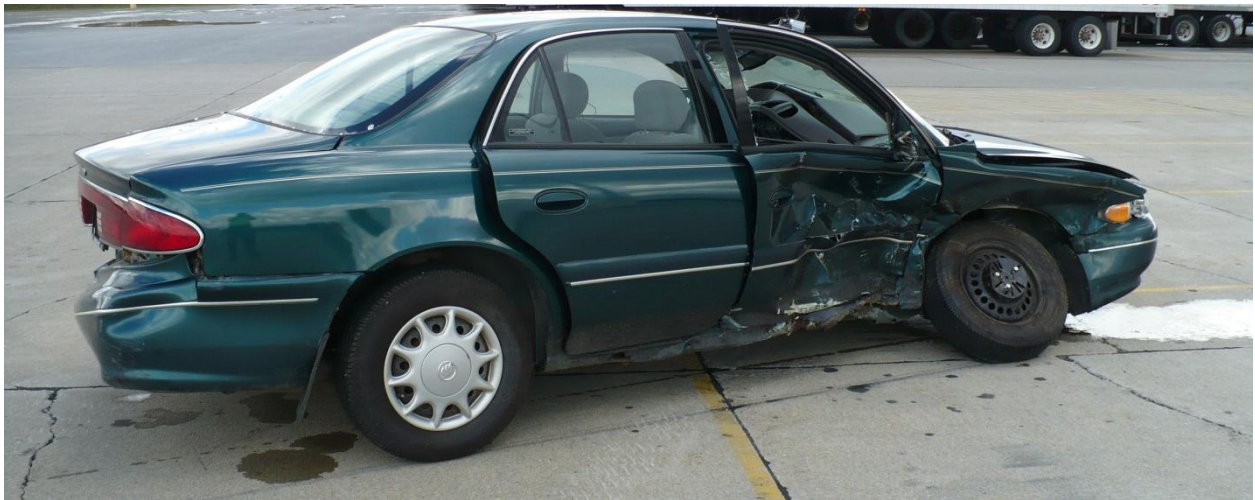
Figure 3: Side damage to the Buick showing the disabled front right wheel.
