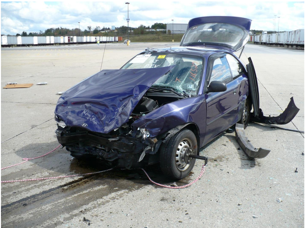
Figure 4: Frontal damage to the Hyundai.
