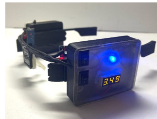
Figure 4. MouseHead - Left view battery and voltage indicator
