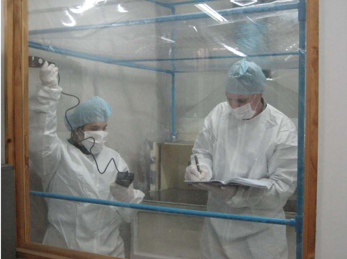
Fig. 5. Measuring particle counts in the cleanroom.
