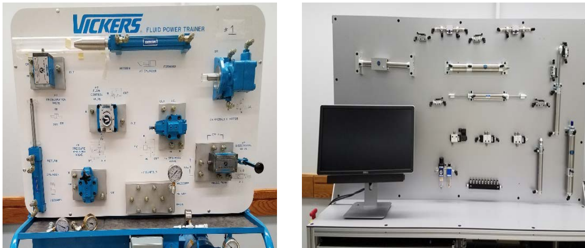
Figure 1. The Hydraulic (left) and pneumatic (right) trainers.
