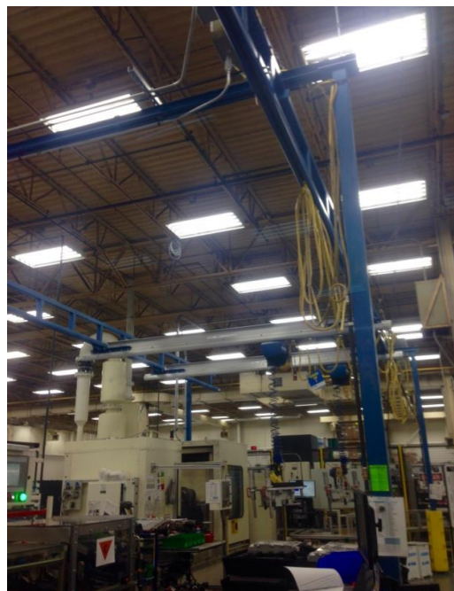
Figure 3: Lift assist structure
