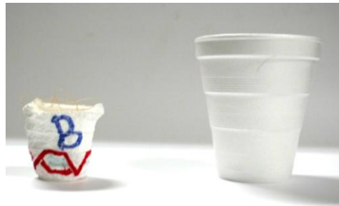
Figure 9: Styrofoam cup that has been submerged in approximately 3,000 meters of water, next to a comparison cup
