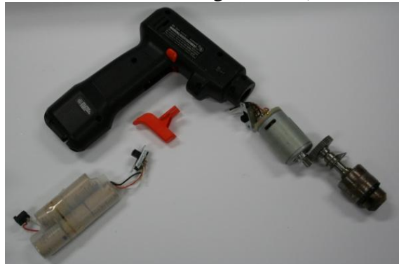
Figure 2: a screwdriver taken apart to reveal its components
