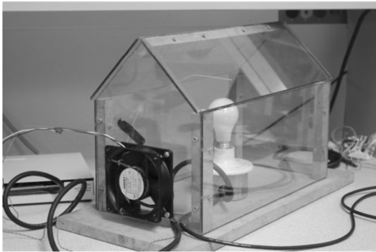
Fig. 3: Physical model of the greenhouse [1]
