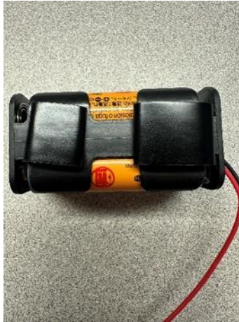
Figure 7. Battery Pack Taping
