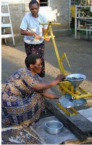
Figure 6. Jatropha nut press in Mali.
