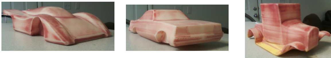
Figure 4: 3D printed scale models. The wheels are excluded for simplicity.
