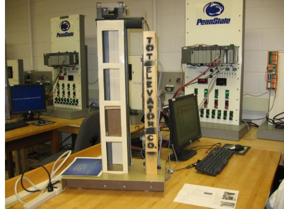
(c) Mix with steel and wood frame and through hole beam sensors
