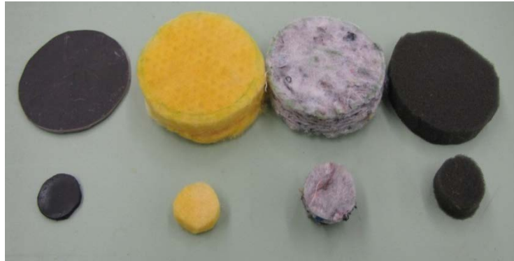
Figure 4: Test specimens used during the validation (From Left to Right: EVA Barrier, Fiberglass insulation, cotton shoddy and Ether Foam)
