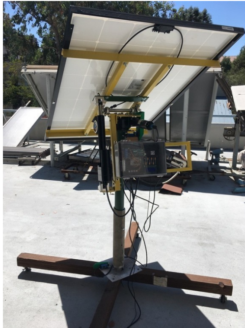
Figure 1: Dual-axis solar tracker built by a senior project team in 2016 [X] with automated controls added by a Summer Undergraduate Research team in 2018.
