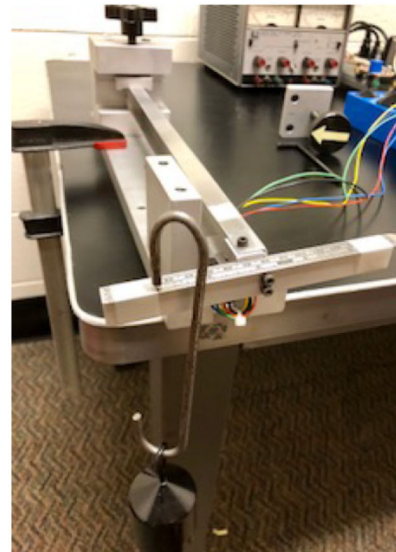
(b) Test with 0.5 kg weight applied to tip crossbar.
