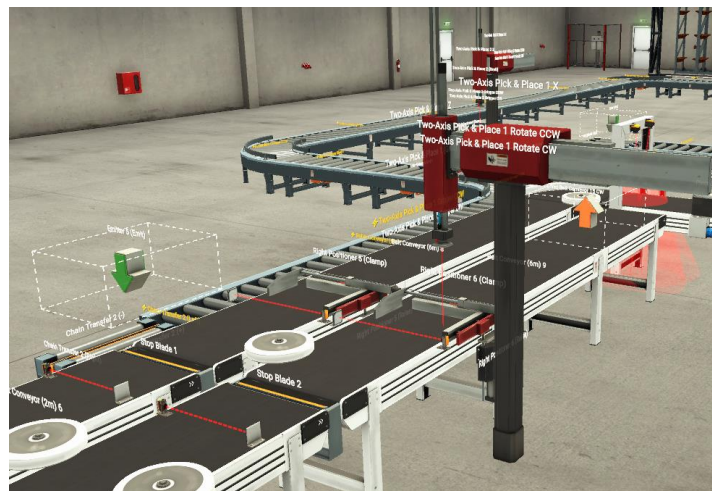
Figure 8: Assembly parts by using the pick and place handling machine
