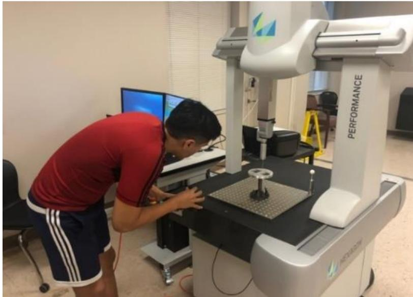
**Fig. 1 Hexagon Global Performance Coordinate Measuring Machine**
