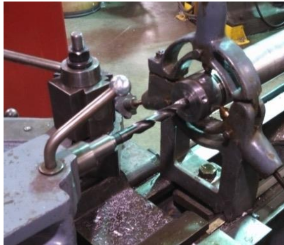
Figure 5. Fixing roller run-out on the drive roller
