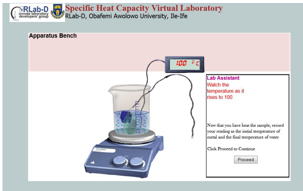
Figure 8: Screen shot showing heating of sample to 100 0 C (Step 8 of the experiment procedure)
